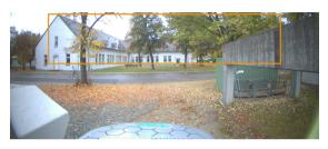
The same scene with different areas of the image used for the internal auto exposure control.
